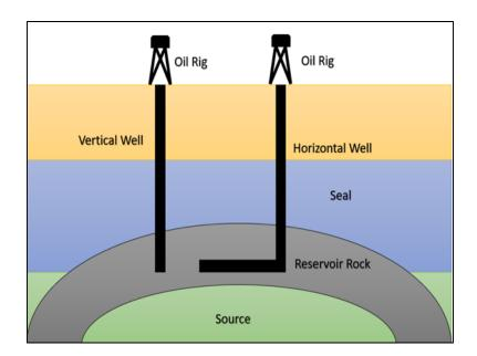
14. For the Vertical Well on the left, we drill straight down until we reach the reservoir where we can produce oil and gas. The Horizontal Well on the right is a well with one or more sections drilled at an angle from the vertical well. There is one other type of well — a directional well — that, broadly speaking, shares certain characteristics of both vertical and horizontal wells. A directional well is simplistically depicted as follows:<sup>2</sup>
