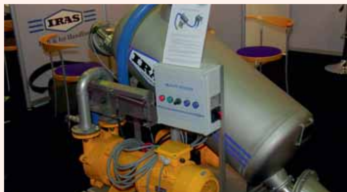
Iras' vacuum pumps can be used to transport fish both dead and alive from 8 m to 2 km. Customers include fish farmers, fishing vessels, and processing factories.
