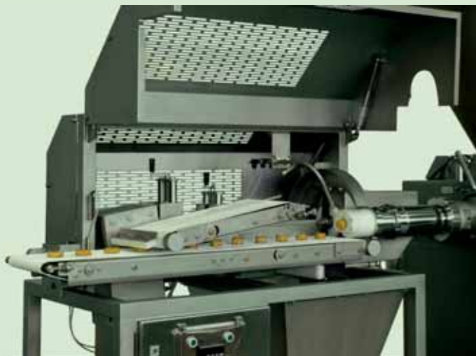
VEMAG's FM 250 produces precisely shaped products from dimensionally stable fish, meat and vegetable materials. Product shapes and sizes can be varied using easily exchangeable nozzles.
