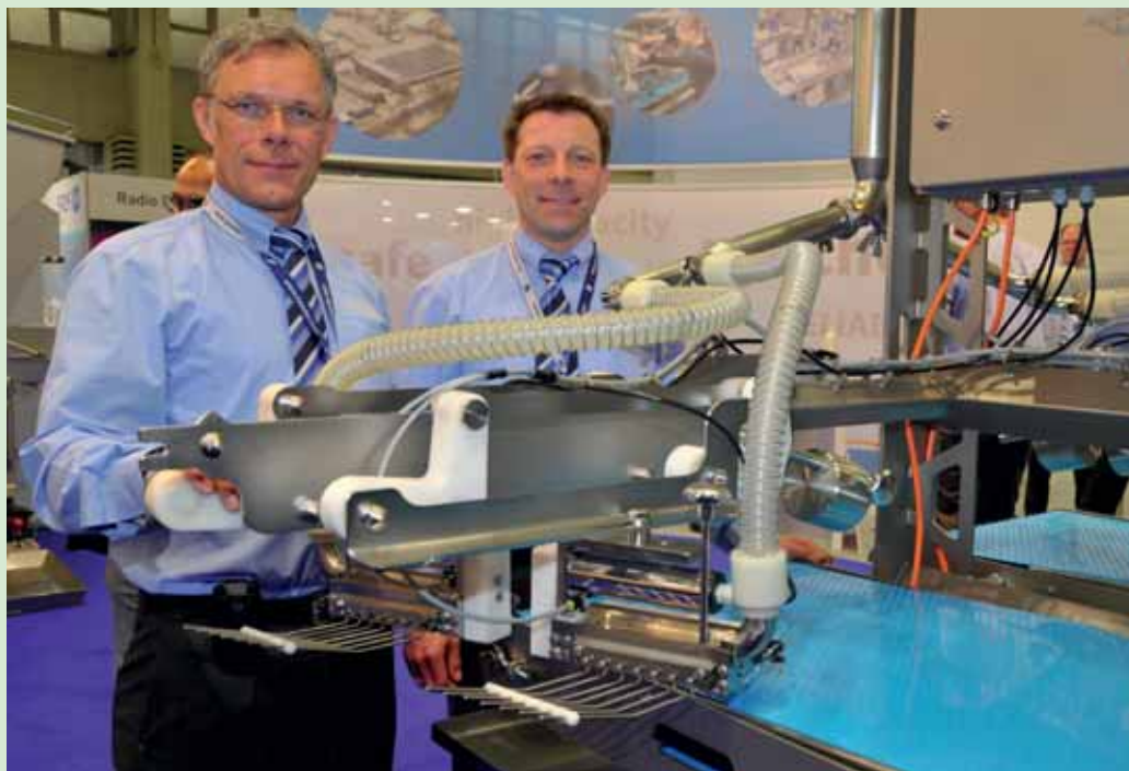
Depending on the size and meat quality of the salmon the Pinbone Remover Baader 867 can remove the pinbones from about 20 fillets per minute.
