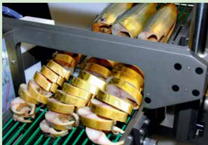
Adjustable cutting angle between 15 and 90°, high slicing performance and a clean cut are features of Salmco's vertical slicer SM 5290.
